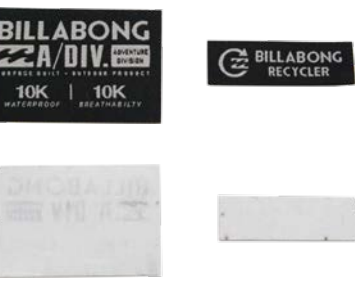
Heat transfer woven label Heat-seal backing Flat Press Dwell time: 15-20 second Dwelling temperature: 160°C-200°C Pressure: 40-60 PSI Laundry test: 30°C temperature machine cold, tumble dry cold
